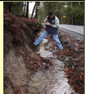
Warren County SWCD Technician Dean Moore using GPS to log roadside ditch erosion around Schroon Lake
